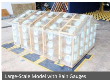
Wind-Driven Rain Test of Full-Scale Model
