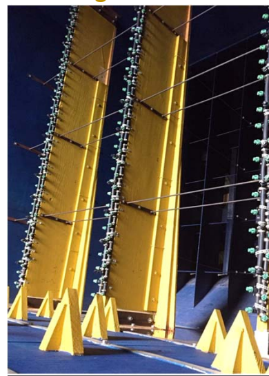
Water-Injection System for Wind-Driven Rain
