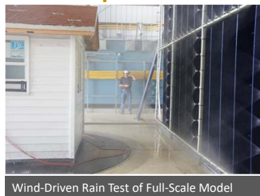
Wind-Driven Rain Test of Full-Scale Model
